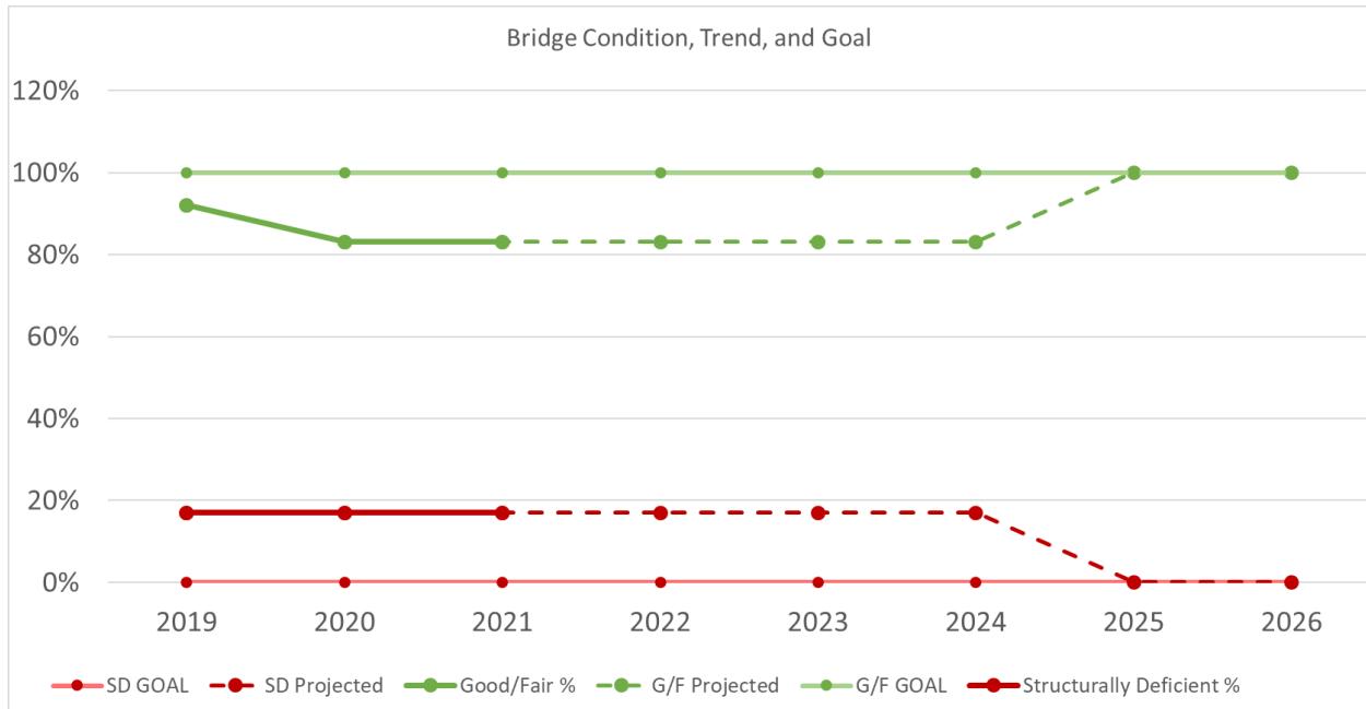
Figure 8: Condition, projected trend, and goal for OCRC's good/fair and structurally deficient bridges
